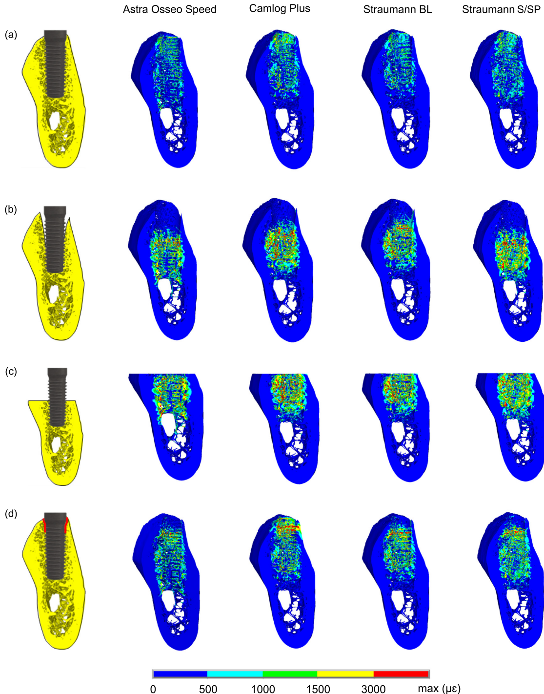
Fig. 6. Differences in strain intensity ( \mu\epsilon ) distribution in the adjacent bone at the bone-implant interface for – (a) full bone bonded, (b) circular bone loss, (c) horizontal bone loss and (d) full bone friction; in the four implants. Schemes in the leftmost column illustrate the bone morphology used in simulating corresponding configurations. The red marker in (d) indicates the region where frictional contact is defined instead of 'bonded always'. For a colour representation, the reader is referred to the online version of this paper. (For interpretation of the references to colour in this figure legend, the reader is referred to the web version of this article.)
