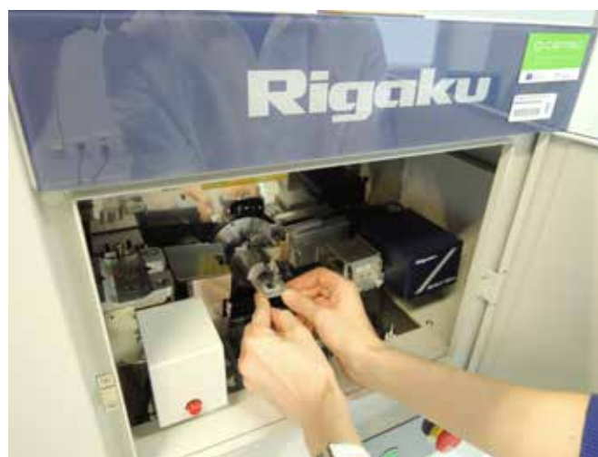
Diffraction chamber of Benchtop with the sample of PA12 and particular diffractograms
