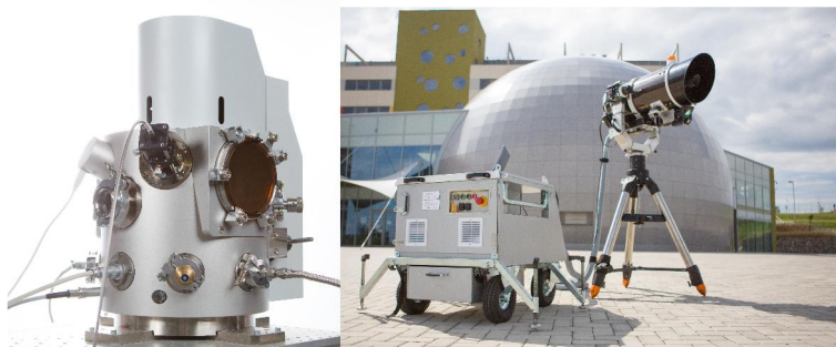
Left: LIBS interaction chamber, right: rLIBS device.
