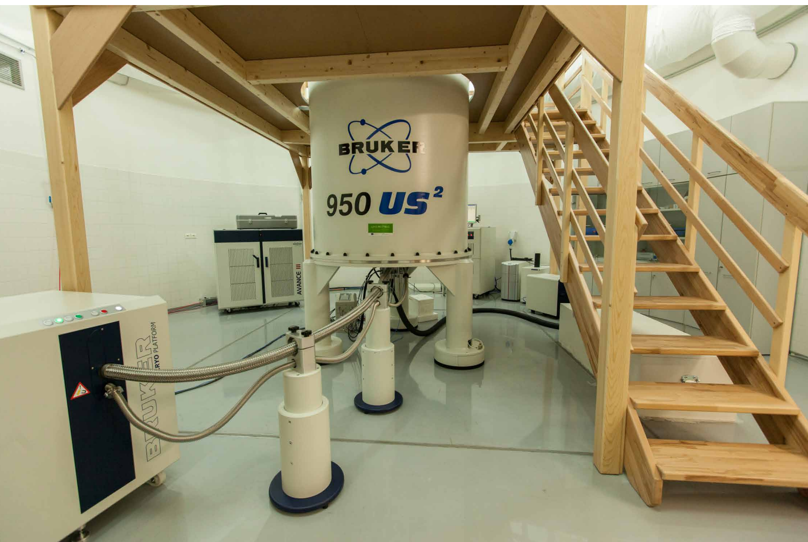
950 MHz NMR spectrometer for high-resolution spectroscopy in liquids
