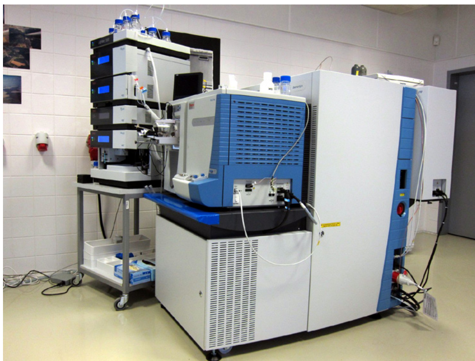
◀ LC-MS/MS system with high resolution mass spectrometer Orbitrap Elite.
