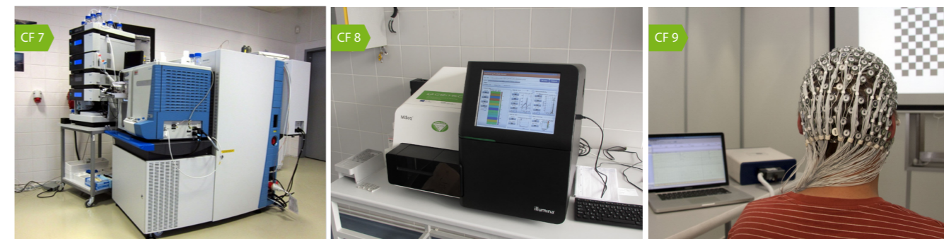
▲ LC-MS/MS system with high resolution mass spectrometer Orbitrap Elite from Proteomics core facility
